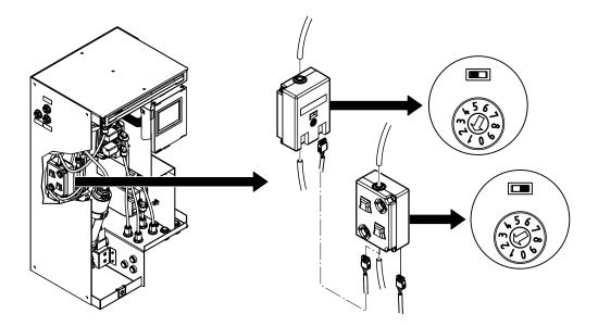
Fig. 85: Replacement of the water sensor module
