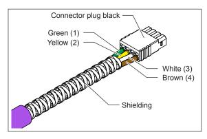
Fig. 28: Connect CAN bus cable
