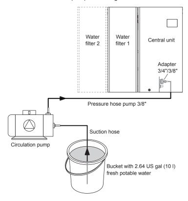
Fig. 73: Schematic diagram for the connection of the circulation pump for flushing
