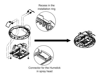
Fig. 25: Fixing the installation ring and catch springs to the spray head
