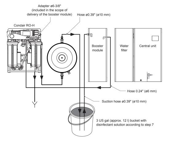
Fig. 79: Schematic diagram of the hose layout for disinfection of the Condair RO-HB for MN systems
