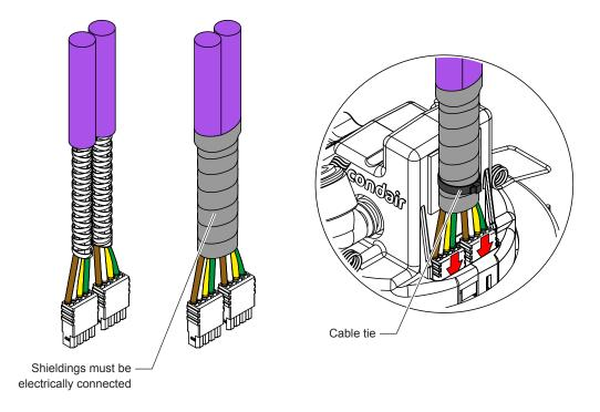
Fig. 31: Connect the CAN bus cable to the spray head
