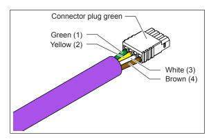
Fig. 46: Connecting the plug(s) to the CAN bus cable(s)
