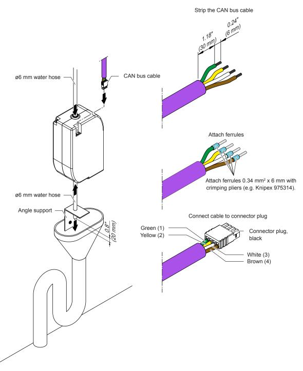
Fig. 36: Connect external drain module
