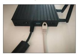
Fig. 59: Connecting the gateway to the in-house network
