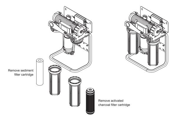
Fig. 77: Removing the activated carbon filter and sediment filter cartridge
