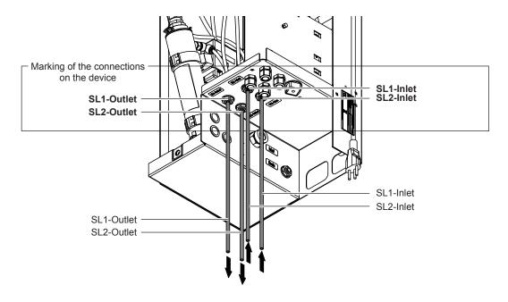
Fig. 40: Connection of the spray loop hoses
