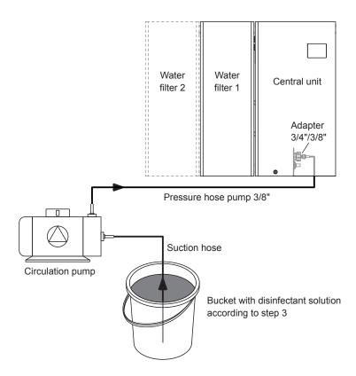
Fig. 71: Schematic diagram for the connection of the circulation pump for disinfection
