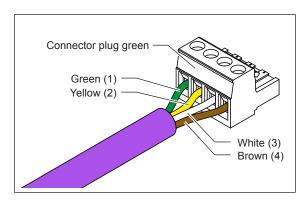
Fig. 44: Connecting the plug(s) to the CAN bus cable(s)
