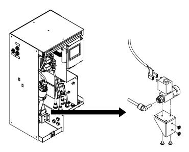
Fig. 94: Replacing the inlet valve
