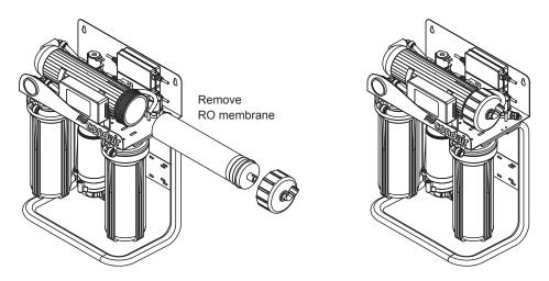
Fig. 78: Removing the RO membrane
