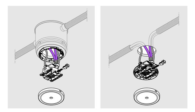
Fig. 100: Replacing the humidity sensor (screwed spray head version on the left, pluggable spray head version on the right)
