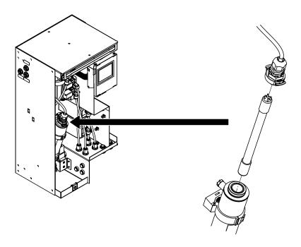
Fig. 67: Replacing the UV lamp in systems produced from April 1, 2020
