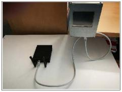
Fig. 60: Connecting the gateway to the ConBox
