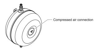
Fig. 84: Compressed air connection expansion tank
