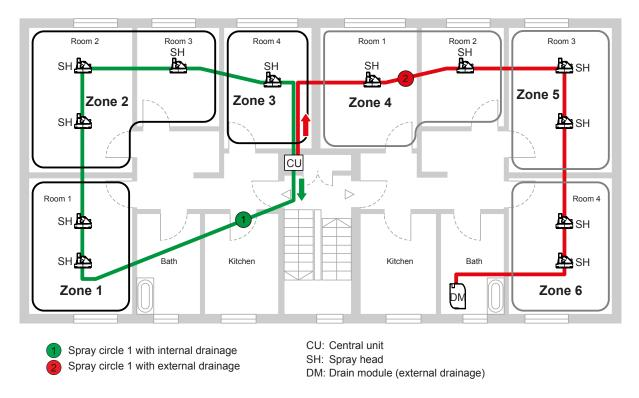
Fig. 6: Spray loop design
