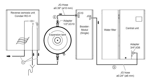
Fig. 49: Connection diagram
