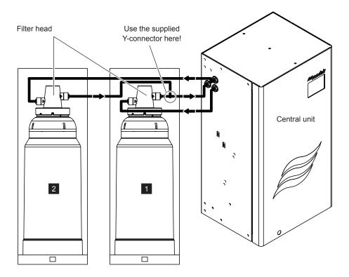
Fig. 39: Connection diagram with two water filters
