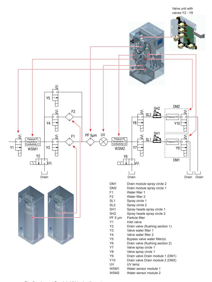
Fig. 5: Layout Condair MN hydraulic system
