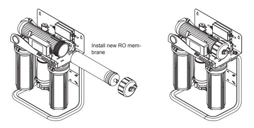
Fig. 82: Installing new RO membrane
