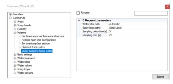
Fig. 65: Flushing spray loops with "Water sampling fluidic paths"
