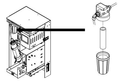
Fig. 68: Replacing the filter cartridge of the particle filter
