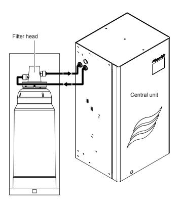
Fig. 38: Connection diagram with one water filter
