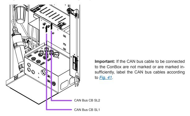
Fig. 41: Insert CAN bus cables to be connected to the ConBox into the central unit
