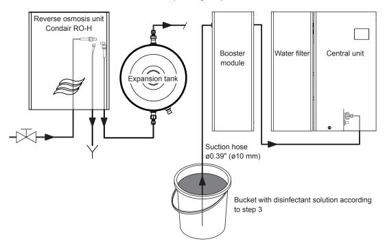
Fig. 72: Schematic diagram of the hose layout for disinfection of MN systems with RO-HB
