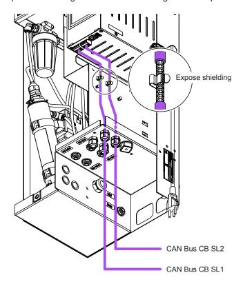
Fig. 47: Connecting CAN bus cables for spray loop 1 and spray loop 2 to the ConBox
