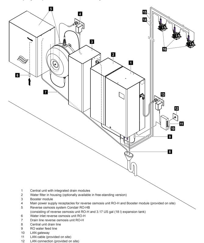
Fig. 2: Overview Condair MN system with one spray loop and internal drainage of the spray loop and reverse osmosis system Condair RO-HB
