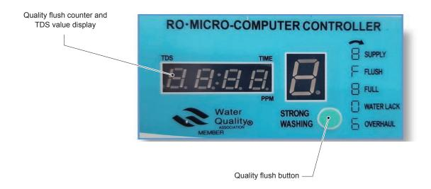
Fig. 83: Display Condair RO-HB controller
