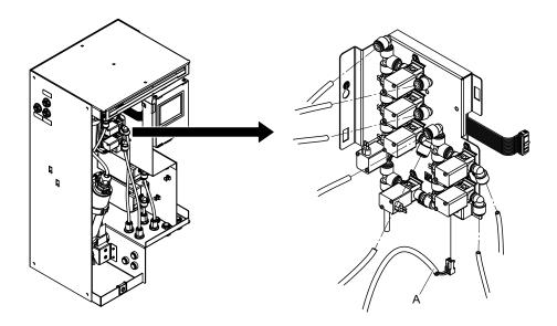
Fig. 91: Replacing the valve block
