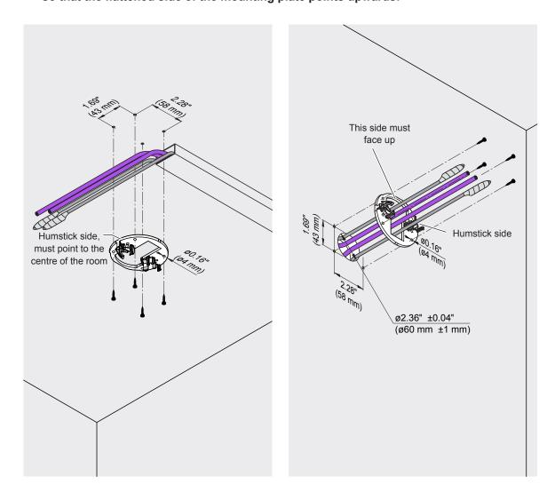
Fig. 26: Mount the installation ring.
