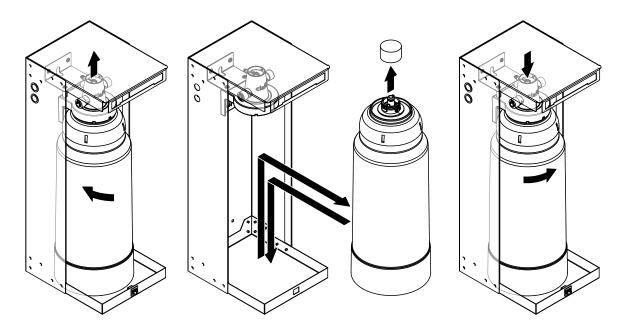
Fig. 69: Replacing the water filter
