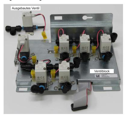
Fig. 92: Removing a valve
