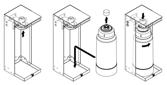
Fig. 37: Installation of the water filter
