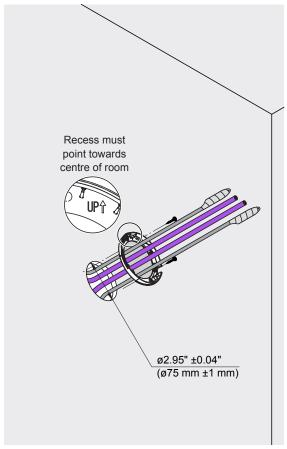
Fig. 24: Mount the installation ring
