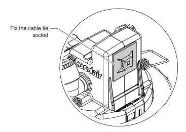
Fig. 30: Fixing the self-adhesive cable tie socket
