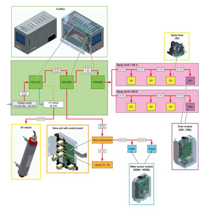
Fig. 7: Electrical diagram Condair MN
