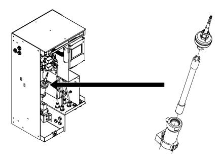
Fig. 66: Replacing the UV lamp in systems produced until March 31, 2020
