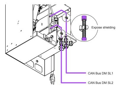
Fig. 48: Connecting CAN bus cables for spray loop 1 and spray loop 2 to the drain modules
