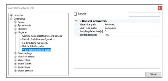
Fig. 57: Flushing spray loops with "Water sampling fluidic paths"
