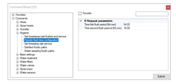
Fig. 55: Setting the periodic flushing time
