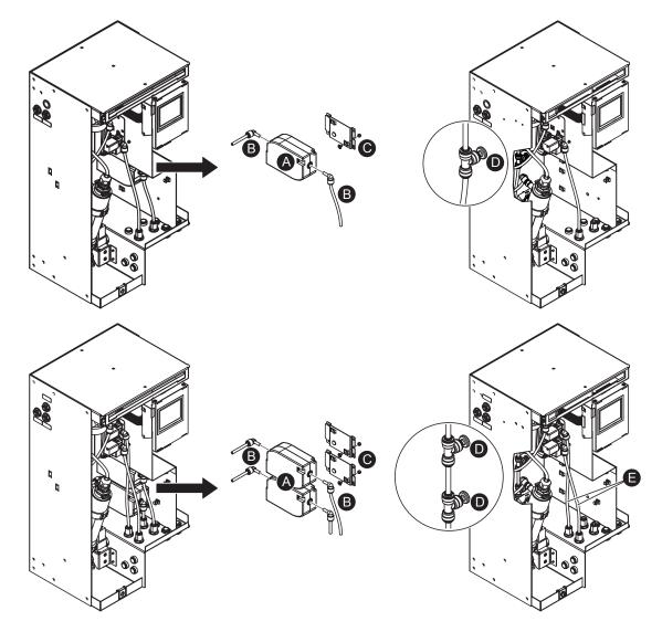
Fig. 34: Removal of the drain modules
