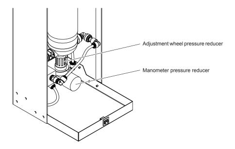
Fig. 56: Pressure reducer booster module
