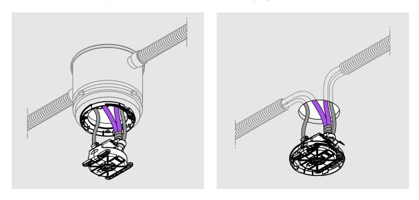
Fig. 29: Connect CAN bus cables and hoses to the spray head
