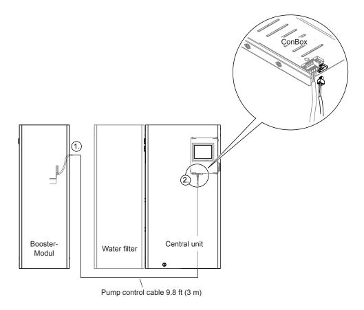
Fig. 50: Connection of the booster module control cable
