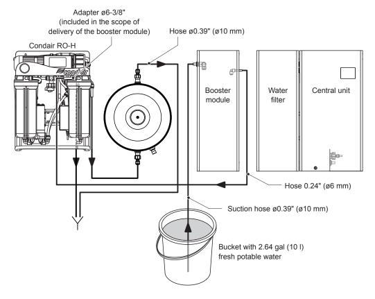
Fig. 80: Schematic diagram of the hose layout for flushing of the Condair RO-HB for MN systems
