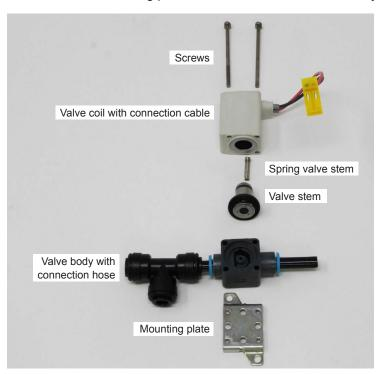
Fig. 93: Dismantling the valve
