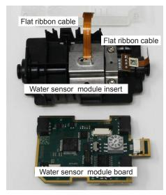
Fig. 86: Dismantling the water sensor module
