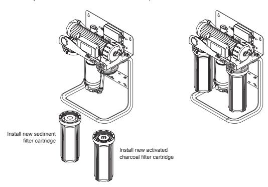
Fig. 81: Installing new activated carbon filter and sediment filter cartridge
