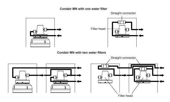
Fig. 70: Remove water filter(s) and join inlet and outlet hoses
