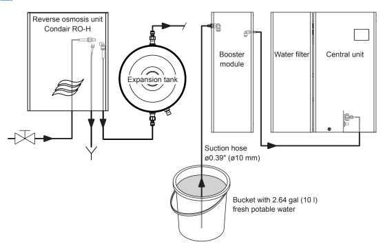
Fig. 74: Schematic diagram of the hose layout for flushing of MN single systems with RO-HB
