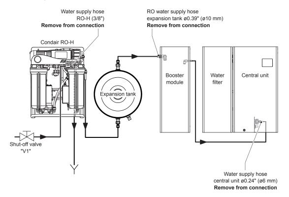
Fig. 76: Removing the hoses
