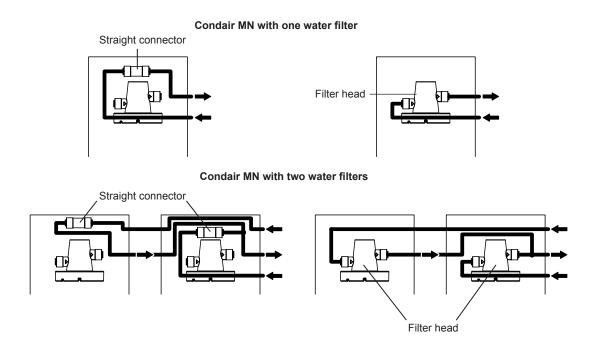
Fig. 75: Connect the inlet and outlet hoses to the filter head(s)
