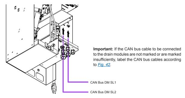
Fig. 42: Insert CAN bus cables to be connected to the drain modules into the central unit
