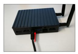
Fig. 58: Connecting the gateway to the power supply
