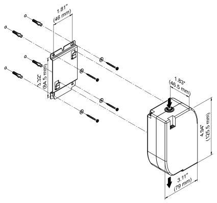
Fig. 35: Installation of the external drain module
