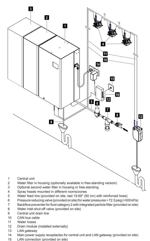
Fig. 3: Overview Condair MN system with one spray loop and external drainage of the spray loop
