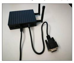
Fig. 62: Connecting the gateway to the laptop using the RS232 cable
