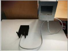
Fig. 63: Connecting the gateway to the ConBox
