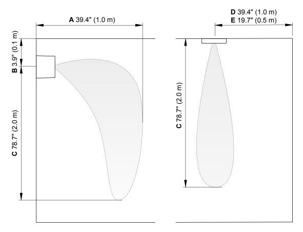
Fig. 15: Required minimum distances in the positioning of spray heads
