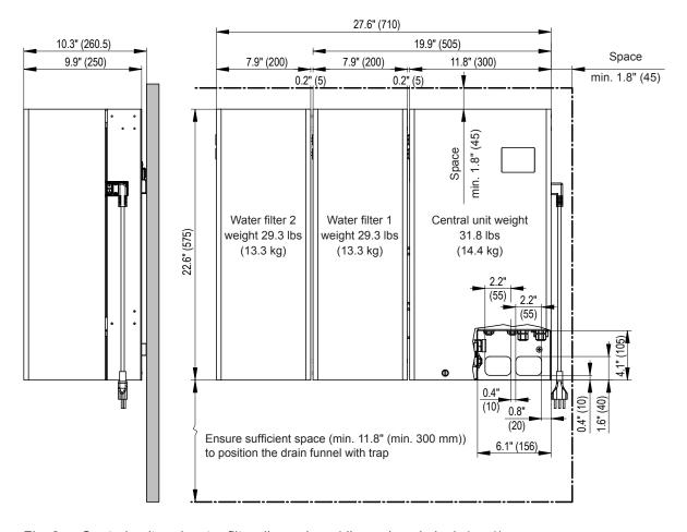
Central unit and water filter dimensions (dimensions in inch (mm))
