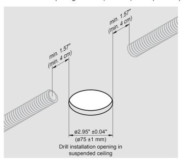
Fig. 21: Drill installation opening in the suspended ceilings
