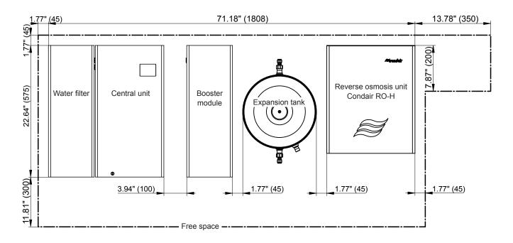
Fig. 13: Placement example 2 (dimensions in inch (mm))
