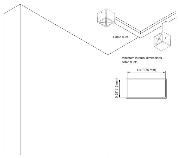
Fig. 23: Laying cable ducts
