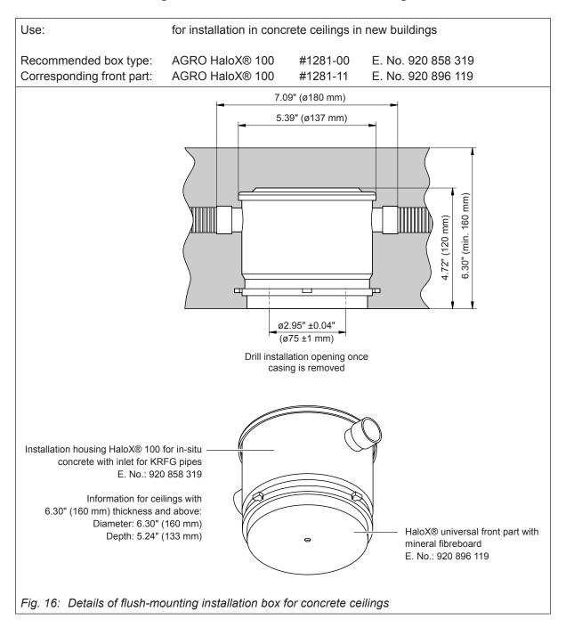
The installation boxes for concrete ceilings must be placed in the intended locations on the shell and attached to the casing.
