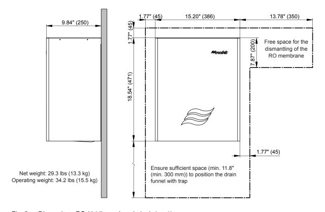
Fig. 9: Dimensions RO-H (dimensions in inch (mm))
