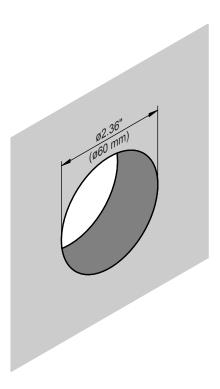
Fig. 22: Drill wall duct(s)
