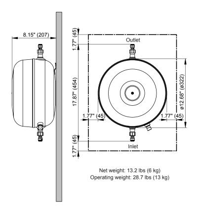
Fig. 10: Dimensions expansion tank (dimensions in inch (mm))
