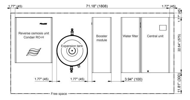
Fig. 12: Placement example 1 (dimensions in inch (mm))
