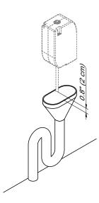
Fig. 27: Installing a drain funnel with trap for external drain module(s)
