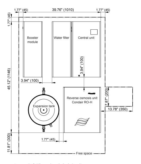
Fig. 14: Placement example 3 (dimensions in inch (mm))
