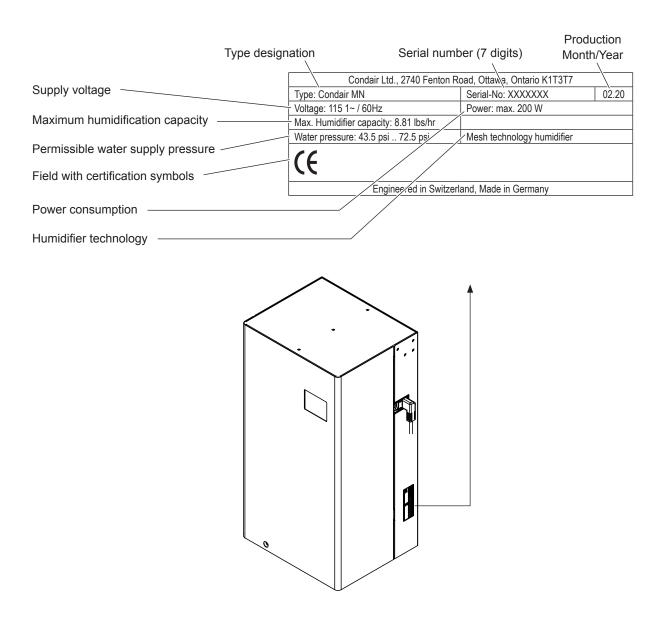
Fig. 1: Location of the specification label
