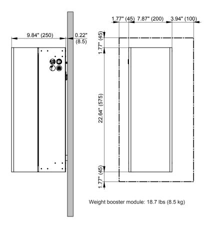
Fig. 11: Dimensions booster module (dimensions in inch (mm))
