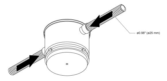
Fig. 17: Details of flush-mounting installation box for concrete ceilings
