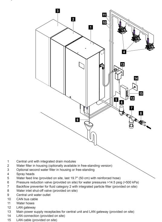
Fig. 2: Overview of Condair MN system with internal drainage of spray circuit
