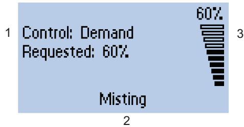
Figure 4 - Ultrasonic Humidifier Home Screen - Single Reservoir
