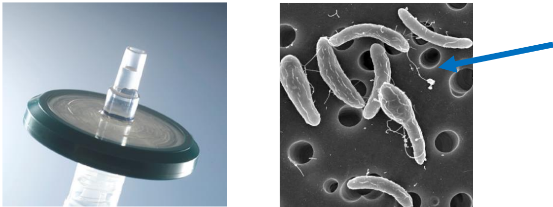
Figure 18 - Filtration of Water and Bacteria on Filter Surface
