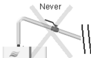
Install a valve or other obstruction
